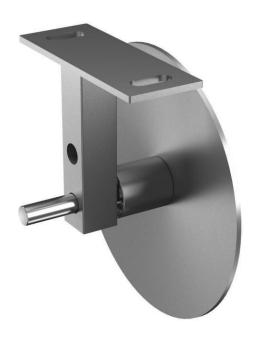
Designed with a smooth conical surface that rotates as the conveyor belt becomes misaligned from the center line, the Side Guide Roller provides protection to conveyor framework as well as providing training action to the conveyor belt.
