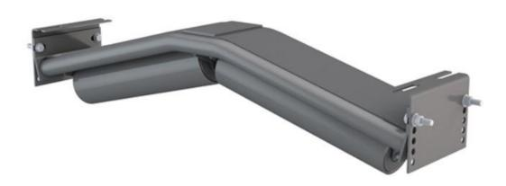
Inverted V-Return (IVR) Idlers are used to positively track the belt on the return side of the conveyor. The PPI IVR is adjustable to increase the displacement and the resulting tracking force on the belt.
