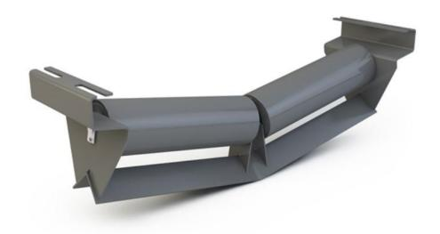
V-Return Idlers are available with 4.5" and 7" drop heights and are built with a 10° two roll trough configuration that allows gravity to naturally keep the belt centered. The shorter two roll design enables the user to implement much lighter rolls than the traditional single roll configurations.
